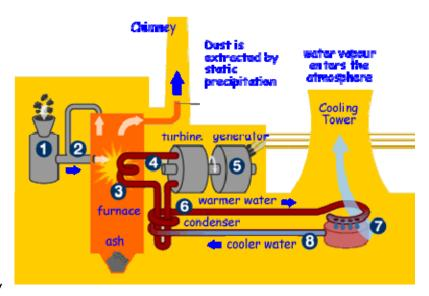
Common energy sources used to power electricity power stations are: the fossil fuels: coal, oil and gas, which are burned to produce heat; biomass which is burned to produce heat (these are smaller scale generally) and uranium/plutonium, in which nuclear fission produces the heat.
